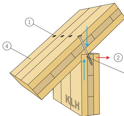
3.3 EAVES DESIGN WITHOUT CANOPY (INDEPENDENT OF PANEL BEARING DIRECTION)
