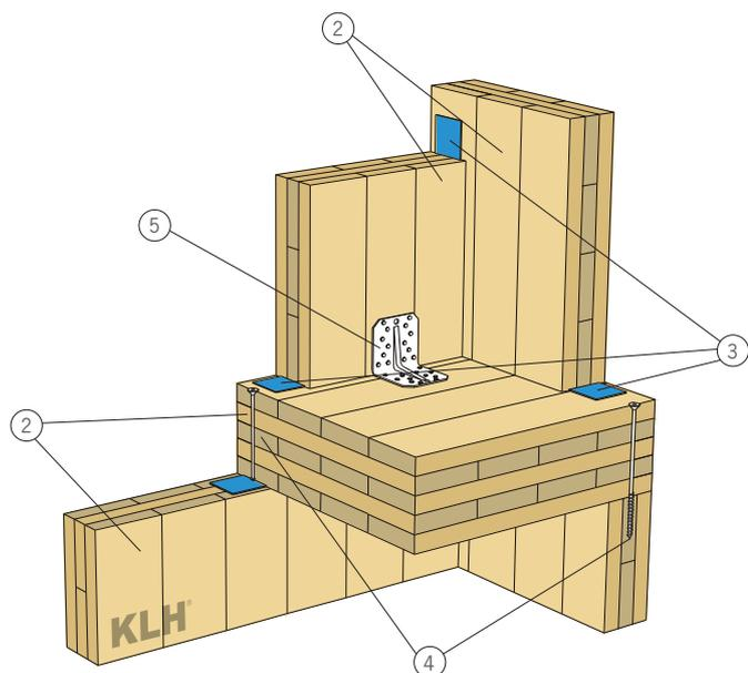
WALL-WALL CONNECTION, ROOF-WALL CONNECTION
