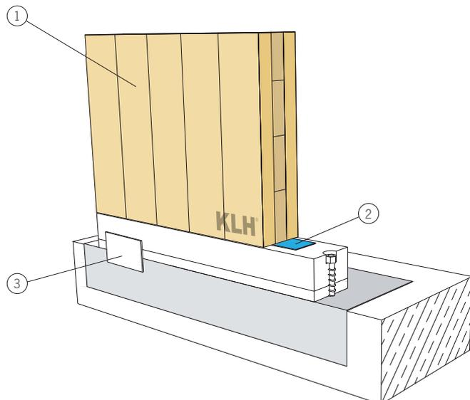
**AIR TIGHTNESS – FLOW-TIGHT CONSTRUCTIONAL DESIGN**
