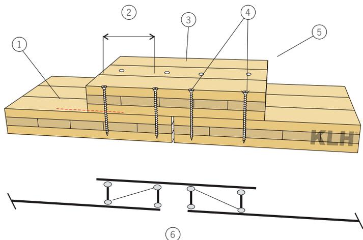
TRANSVERSE CEILING JOINTS, FLEXIBLE AND BEND-RESISTANT
